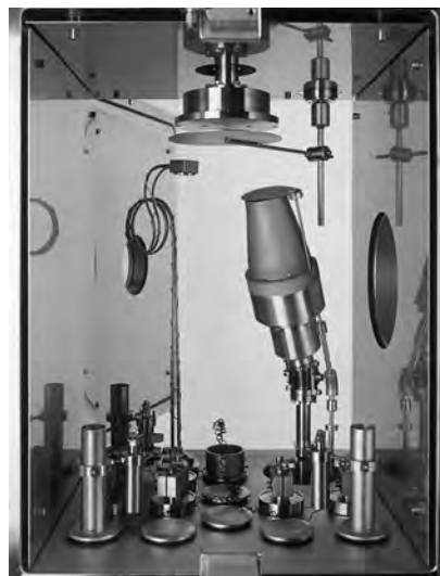
View through the vacuum chamber: front sliding door and rear swivelling door open Design example with sputter source (right) and heated substrate table (top)
