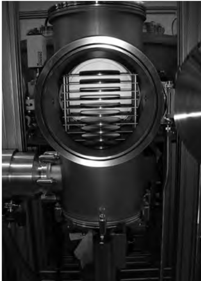
Manually operated load lock chamber with substrate magazine
