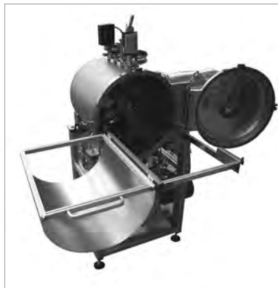
Opened coating chamber with retracted substrate receiver
