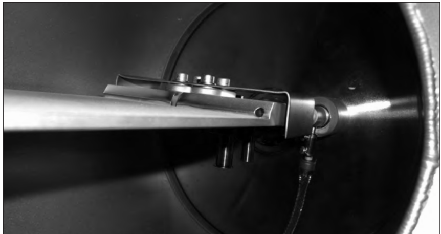
Insulated substrate fork with RF bias connection
